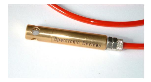
The sensors use optoelectronic detection of a reversible optical change that is induced by oils, hydrocarbons and liquid fats, but not by any water or other "hydrophilic" liquids that may be present. They can be monitored by connection to a telemetry system or via mobile phone or other wireless networks.
